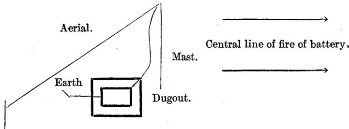
In future all stations will be erected on this principle—i. e., mast toward the target. Dugout and lead at mast end of aerial.
