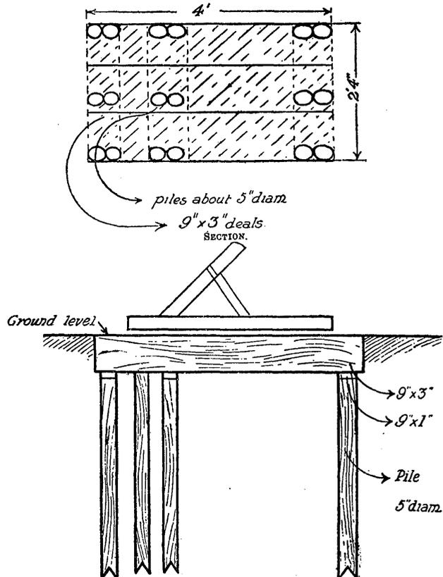
The piles are driven in vertically a maximum distance of 4', the distance depending on state of ground and resistance offered. The tops are then cut off level.
